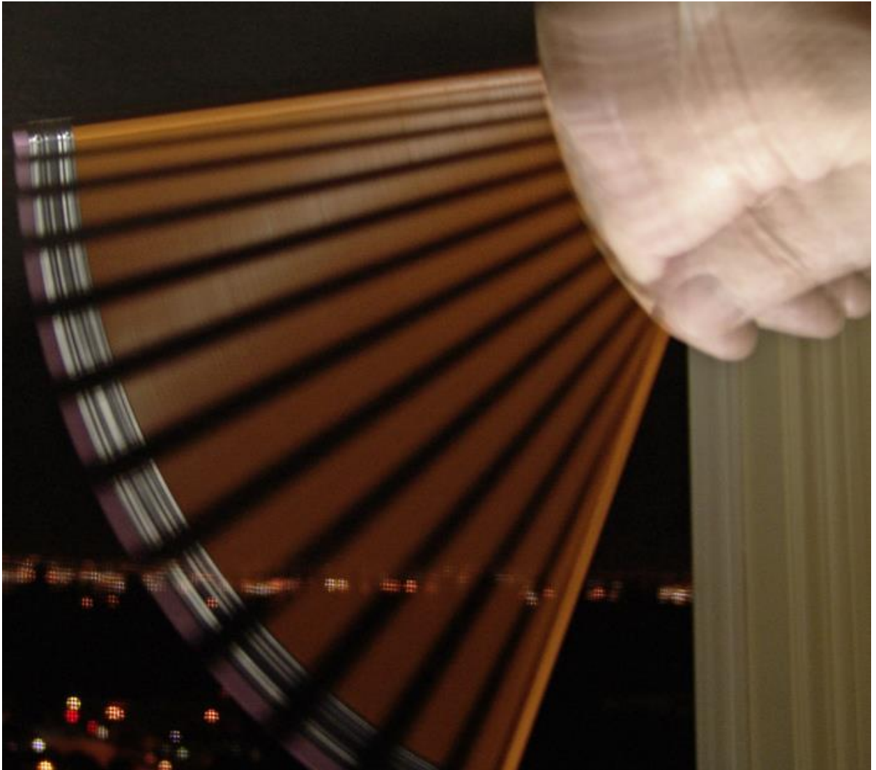
Figure 2. Stroboscopic effect from a moving pencil in front of a light source with a flicker index of 0.34
