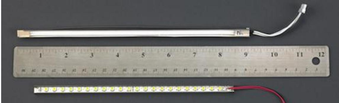
**Fig 1.** CCFL tube BLUs (top) are rapidly giving way to LED strings or rails (bottom) for LCD backlighting.
